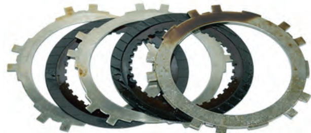
Automatic transmission clutch plates after cleanup with AMSOIL Engine and Transmission Flush reveal lighter glazing and varnish.
