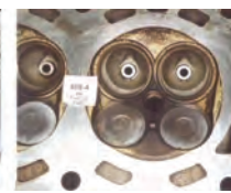
Combustion chamber after P.i. treatment.
