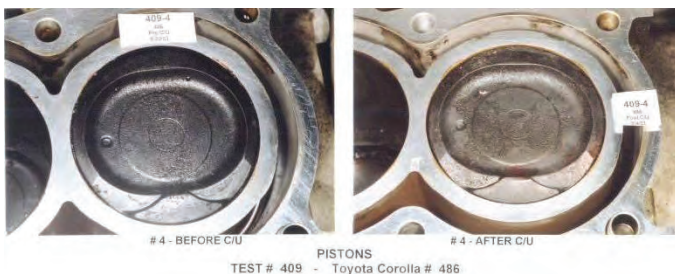
Picture G - Piston before P.i. treatment
