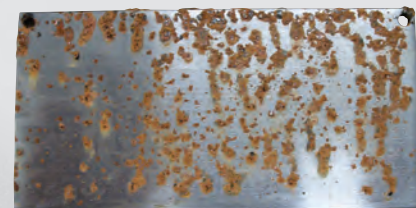
After 192 hours in a humidity cabinet, the metal coupon treated with a leading competitive product rusted severely.
