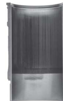
Severely Scuffed Liner
